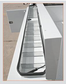
Available on Streetside, Streetside and Curbside or none. Incabinet latch for security. Includes gas strut openers, adjustable dividers and stainless steel hinges. (Model 1440 only)
