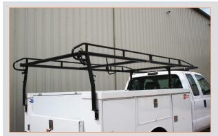
KargoMaster Pipe and Ladder Racks are available for both 1440 and 2240 service bodies. Racks are built with 2" Dia. x .083" steel tube and have a 1700 lb capacity. 62" load space is the widest available. High gloss black marine grade powder coat specially formulated to resist corrosion and abrasion. Will fit on bodies with and without fliptops. Additional accessories available.
