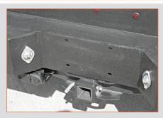
Bolt on step bumper with black lava powder coat and 2 vise sockets. Receiver hitch is independent from bumper and mounted directly to chassis. LED stop/turn/tail lights.
