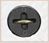
4 hidden deck tiedowns with pull up loops. Tiedowns are flush with floor when not in use. 3500 lb rated pull capacity.
